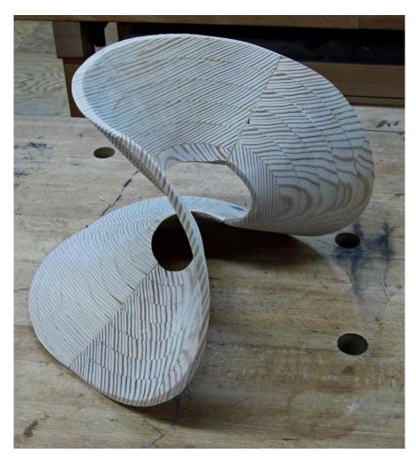
**Tom** described this adventure by noting that each of the curved segments was made by scroll sawing concentric rings with beveled edges, which when glued together formed segments of curved, somewhat conical surfaces. Joining these segments together edge-to-edge, produced the complex shape of the Mobius. Lots of sanding was required......!
